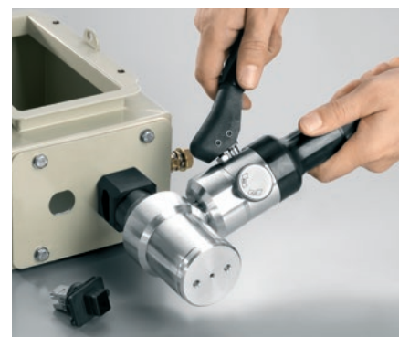
Punching out holes for a variety of industrial Ethernet connectors.
